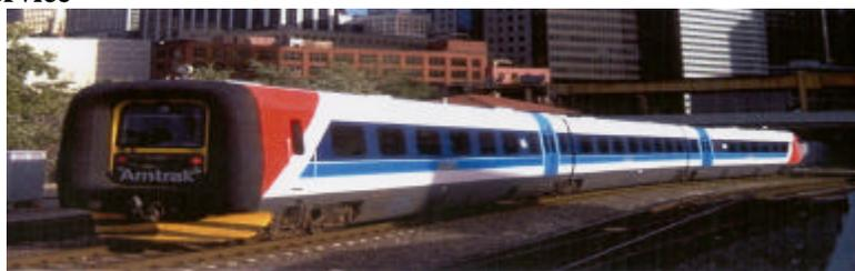
**Adtranz Flexliner IC3 Diesel Multiple Unit (DMU)**
