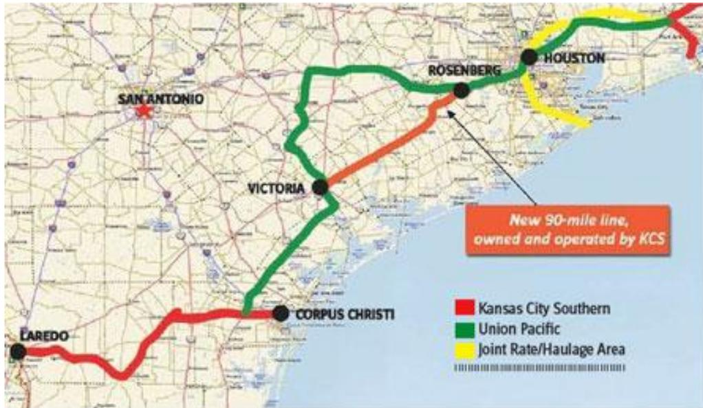
Figure 3-13: New KCS Line Between Rosenberg and Victoria, Texas<sup>9</sup>
